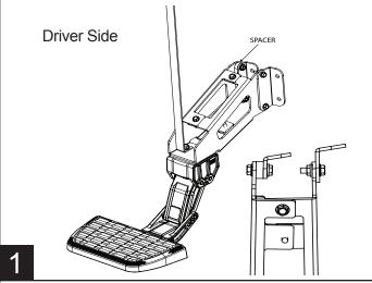
Main Bracket Assembly...On Driver side, bolt Left Main Bracket (3) over Right Main Bracket (4) and hand tighten all three (9) Small M8 Bolts (2 on top, 1 on bottom).
