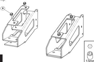
L Bracket Assembly... On Driver Side, bolt spacer in between Left Main Bracket (3) and L Bracket (6) using longer M8 bolts (8). Bolt Right Main Bracket (4) to L Bracket (5) using 2 M8 bollts. Tighten to 20 ft lbs.
